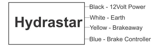
Use a 12 Volt battery source, isolate the wires from the Hydrastar when conducting the BATTERY Test
